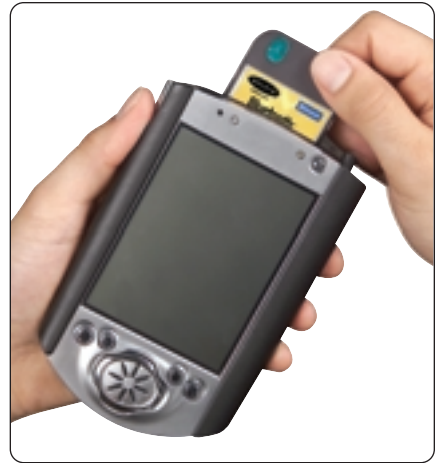
Fig. 7—Inserting the Adapter Card
